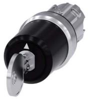
Key-operated switch BKS, 22 mm, round, metal, shiny, lock number S1, with 2 keys, 3 switch positions I-O<II, left latching, right momentary contact type, actuating angle  $2x45^{\circ}$ , 10:30h/12h/13:30h, Key removal I
