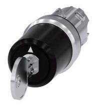
Key-operated switch BKS, 22 mm, round, metal, shiny, lock number S1, with 2 keys, 3 switch positions I-O<II, left latching, right momentary contact type, actuating angle  $2x45^{\circ}$ , 10:30h/12h/13:30h, Key removal O
