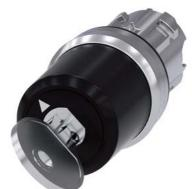
Key-operated switch BKS, 22 mm, round, metal, shiny, lock number S1, with 2 keys, 2 switch positions O-I, latching, actuating angle 90°, 10:30h/13:30h, Key removal I
