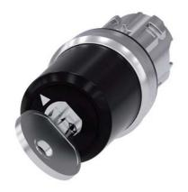
key-operated switch Siemens, 22 mm, round, metal, shiny, lock no. STGH10, with 2 keys, 2 switch positions O-I, latching, actuating angle 90°, 10:30h/13:30h, key removal O+I
