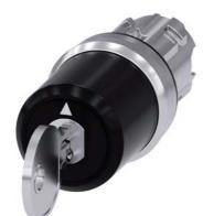
key-operated switch Siemens, 22 mm, round, metal, shiny, lock number SSG10, with 2 keys, 3 switch positions I>O<II, momentary contact on the left, latching on the right, actuating angle 2x45°, 10:30h/12h/13:30h, key removal O+II
