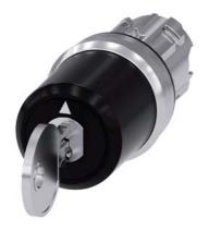
key-operated switch Siemens, 22 mm, round, metal, shiny, lock number SSG10, with 2 keys, 3 switch positions I>O<II, momentary contact on the left, latching on the right, actuating angle  $2x45^{\circ}$ , 10:30h/12h/13:30h, key removal II
