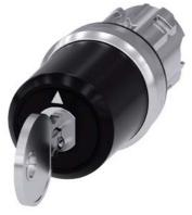
key-operated switch Siemens, 22 mm, round, metal, shiny, lock number SSG10, with 2 keys, 3 switch positions I-O<II, left latching, momentary contact type on the right, actuating angle 2x45°, 10:30h/12h/13:30h, key removal I
