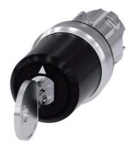
key-operated switch Siemens, 22 mm, round, metal, shiny, lock number SSG10, with 2 keys, 3 switch positions I>O<II, momentary contact type, actuating angle 2x45°, 10:30h/12h/13:30h, key removal O
