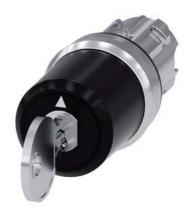
key-operated switch Siemens, 22 mm, round, metal, shiny, lock number SSG10, with 2 keys, 3 switch positions I-O-II, latching, actuating angle 2x45°, 10:30h/12h/13:30h, key removal I+II
