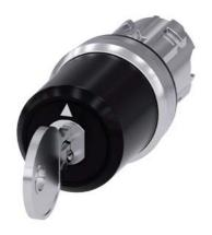
key-operated switch Siemens, 22 mm, round, metal, shiny, lock number SSG10, with 2 keys, 3 switch positions I-O-II, latching, actuating angle  $2x45^\circ,\,10:30h/12h/13:30h,$  key removal II
