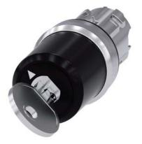
key-operated switch Siemens, 22 mm, round, metal, shiny, lock number SSG10, with 2 keys, 2 switch positions O-I, latching, actuating angle  $90^\circ$ , 10:30h/13:30h, key removal O
