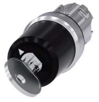
key-operated switch Siemens, 22 mm, round, metal, shiny, lock number SSG10, with 2 keys, 2 switch positions O<I, momentary contact type, actuating angle 45°, 10:30h/12h, key removal O
