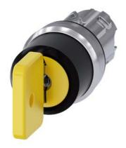
Key-operated switch O.M.R, 22 mm, round, metal, shiny, lock number 73033, yellow, with 2 keys, 3 switch positions I>O<II, momentary contact on the left, latching on the right, actuating angle  $2x45^{\circ}$ , 10:30h/12h/13:30h, key removal II
