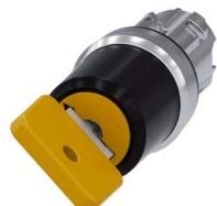
Key-operated switch O.M.R, 22 mm, round, metal, shiny, lock number 73033, yellow, with 2 keys, 2 switch positions O-I, latching, actuating angle  $90^{\circ}$ , 10:30h/13:30h, Key removal I
