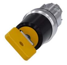
Key-operated switch O.M.R, 22 mm, round, metal, shiny, lock number 73033, yellow, with 2 keys, 2 switch positions O-I, latching, actuating angle  $90^\circ,\,10:30h/13:30h,\,Key\,removal\,O+I$
