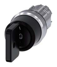
Key-operated switch O.M.R, 22 mm, round, metal, shiny, lock number 73034, black, with 2 keys, 3 switch positions I-O-II, latching, actuating angle  $2x45^\circ,\,10:\!30h/12h/13:\!30h,$  Key removal I+O+II
