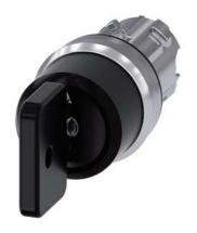
Key-operated switch O.M.R, 22 mm, round, metal, shiny, lock number 73034, black, with 2 keys, 3 switch positions I-O-II, latching, actuating angle  $2x45^\circ,\,10:\!30h/12h/13:\!30h,$  Key removal O
