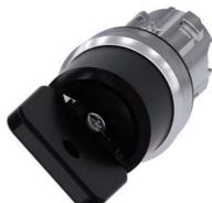
Key-operated switch O.M.R, 22 mm, round, metal, shiny, lock number 73034, black, with 2 keys, 2 switch positions O-I, latching, actuating angle  $90^{\circ}$ , 10:30h/13:30h, Key removal I
