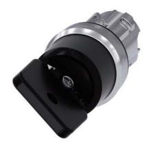
Key-operated switch O.M.R, 22 mm, round, metal, shiny, lock number 73034, black, with 2 keys, 2 switch positions O-I, latching, actuating angle  $90^\circ$ , 10:30h/13:30h, Key removal O+I
