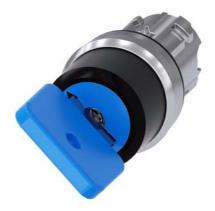
Key-operated switch O.M.R, 22 mm, round, metal, shiny, lock number 73038, blue, with 2 keys, 2 switch positions O-I, latching, actuating angle  $90^\circ$ , 10:30h/13:30h, Key removal O+I
