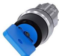
Key-operated switch O.M.R, 22 mm, round, metal, shiny, lock number 73038, blue, with 2 keys, 2 switch positions O<I, momentary contact type, Actuating angle 45°, 10:30h/12h, Key removal O
