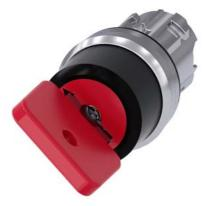
Key-operated switch O.M.R, 22 mm, round, metal, shiny, lock number 73037, red, with 2 keys, 2 switch positions O-I, latching, actuating angle  $90^\circ$ , 10:30h/13:30h, Key removal I
