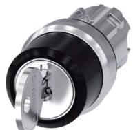
RONIS key-operated switch, 22 mm, round, metal, shiny, lock number 455, with 2 keys, 3 switch positions I-O-II, latching, actuating angle  $2x45^{\circ}$ , 10:30h/12h/13:30h, Key removal I+O+II
