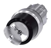
RONIS key-operated switch, 22 mm, round, metal, shiny, lock number 455, with 2 keys, 2 switch positions O-I, latching, actuating angle 90°, 10:30h/13:30h, Key removal I
