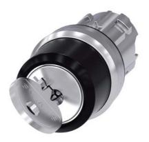
RONIS key-operated switch, 22 mm, round, metal, shiny, lock number 455, with 2 keys, 2 switch positions O-I, latching, actuating angle 90°, 10:30h/13:30h, Key removal O+I
