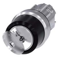
RONIS key-operated switch, 22 mm, round, metal, shiny, lock number 455, with 2 keys, 2 switch positions O<I, momentary contact type, Actuating angle  $45^\circ,\,$  10:30h/12h, Key removal O
