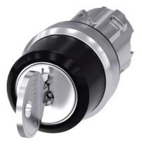
RONIS key-operated switch, 22 mm, round, metal, shiny, lock number SB30, with 2 keys, 3 switch positions I-O<II, left latching, right momentary contact type, actuating angle  $2x45^{\circ}$ , 10:30h/12h/13:30h, key removal I, possible special locks: SB31, 421, 455
