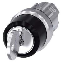
RONIS key-operated switch, 22 mm, round, metal, shiny, lock number SB30, with 2 keys, 3 switch positions I-O<II, left latching, right momentary contact type, actuating angle  $2x45^{\circ}$ , 10:30h/12h/13:30h, key removal O, possible special locks: SB31, 421, 455
