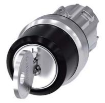
RONIS key-operated switch, 22 mm, round, metal, shiny, lock number SB30, with 2 keys, 3 switch positions I-O-II, latching, actuating angle  $2x45^{\circ}$ , 10:30h/12h/13:30h, key removal O+I, possible special locks: SB31, 421, 455
