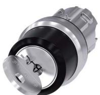
RONIS key-operated switch, 22 mm, round, metal, shiny, lock number SB30, with 2 keys, 2 switch positions O-I, latching, actuating angle 90°, 10:30h/13:30h, key removal O+I, possible special locks: SB31, 421, 455
