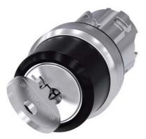
RONIS key-operated switch, 22 mm, round, metal, shiny, lock number SB30, with 2 keys, 2 switch positions O<I, momentary contact type, Actuating angle  $45^\circ, 10:30h/12h,$  key removal O, possible special locks: SB31, 421, 455
