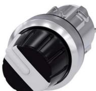
Selector switch, 22 mm, round, metal, shiny, white, Rotary knob, 4 switch positions I-II-III-IV, latching, Actuating angle  $4x90^\circ,$  3h/6h/9h/12h
