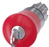
EMERGENCY STOP mushroom pushbutton, 22 mm, round, metal, shiny, red, 40 mm, with RONIS lock, lock number 455, positive latching, acc. to EN ISO 13850, key-operated release
