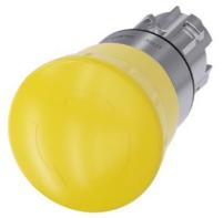
Mushroom pushbutton, 22 mm, round, metal, shiny, yellow, 40 mm, positive latching, acc. to EN ISO 13850, rotate-to-unlatch
