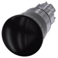
Mushroom pushbutton, 22 mm, round, metal, shiny, black, 40 mm, positive latching, acc. to EN ISO 13850, rotate-to-unlatch
