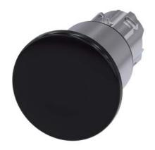
Mushroom pushbutton, 22 mm, round, metal, shiny, black, 40 mm, 3 switch positions, latches after pushing in, unlatches by pull-to-unlatch mechanism to center position, after pulling out the button Retraction to center position
