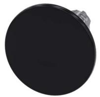
Mushroom pushbutton, 22 mm, round, metal, shiny, black, 60 mm, latching, Pull-to-unlatch mechanism
