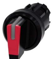
Selector switch, illuminable, 22 mm, round, plastic, red, selector switch, short, 3 switch positions I>O<II, momentary contact on the left, latching on the right, actuating angle  $2x45^{\circ}$ , 10:30h/12h/13:30h
