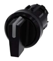
Illuminable selector switch, 22 mm, round, plastic, black, Selector switch short, 3 switch positions I>O<II, momentary contact on the left, latching on the right, actuating angle  $2x45^{\circ}$ , 10:30h/12h/13:30h
