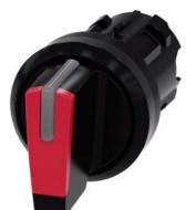
Selector switch, illuminable, 22 mm, round, plastic, red, selector switch, short, 3 switch positions I-O<II, left latching, right momentary contact type, actuating angle  $2x45^{\circ}$ , 10:30h/12h/13:30h
