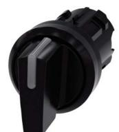
llluminable selector switch, 22 mm, round, plastic, black, Selector switch short, 3 switch positions I-O<II, left latching, right momentary contact type, actuating angle  $2x45^{\circ}$ , 10:30h/12h/13:30h
