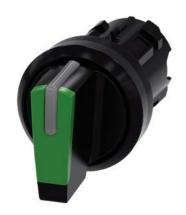
Selector switch, illuminable, 22 mm, round, plastic, green, selector switch, short, 3 switch positions I>O<II, momentary contact type, actuating angle 2x45°, 10:30h/12h/13:30h
