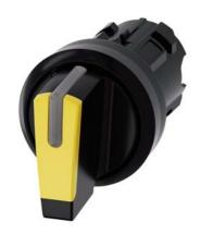
Selector switch, illuminable, 22 mm, round, plastic, yellow, selector switch, short, 3 switch positions I>O<II, momentary contact type, actuating angle  $2x45^{\circ}$ , 10:30h/12h/13:30h
