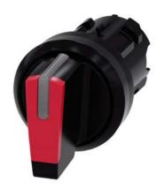
Selector switch, illuminable, 22 mm, round, plastic, red, selector switch, short, 3 switch positions I>O<II, momentary contact type, actuating angle  $2x45^{\circ}$ , 10:30h/12h/13:30h
