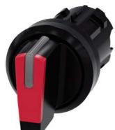
Selector switch, illuminable, 22 mm, round, plastic, red, selector switch, short, 3 switch positions I-O-II, latching, actuating angle  $2x45^\circ$ , 10:30h/12h/13:30h
