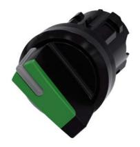
Selector switch, illuminable, 22 mm, round, plastic, green, selector switch, short, 2 switch positions O-I, latching, actuating angle  $90^\circ$ , 10:30h/13:30h
