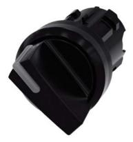
Illuminable selector switch, 22 mm, round, plastic, black, Selector switch short, 2 switch positions O-I, latching, actuating angle  $90^\circ,\,10:30h/13:30h$
