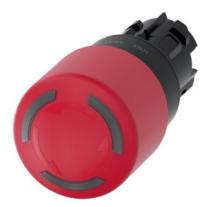
EMERGENCY STOP mushroom pushbutton, illuminable, 22 mm, round, plastic, red, 30 mm, positive latching, acc. to EN ISO 13850, rotate-to-unlatch
