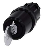
Key-operated switch BKS, 22 mm, round, plastic, Lock No. E9 (VW), without key, 3 switch positions I-O-II, latching, actuating angle 2x45°, 10:30h/12h/13:30h, Key removal I+O+II
