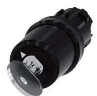
Key-operated switch BKS, 22 mm, round, plastic, Lock No. E9 (VW), without key, 2 switch positions O-I, latching, actuating angle  $90^{\circ}$ , 10:30h/13:30h, Key removal O+I
